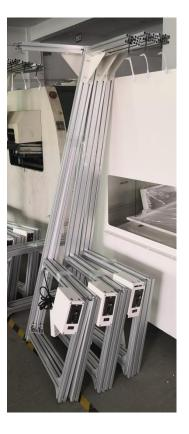
2. Install main table: The aluminum bracket with the foot cup is placed at both ends, and the main plate is placed on the aluminum bracket, and fixed by a triangular plate and a screw, and three triangular plates are used together with the governor box.
