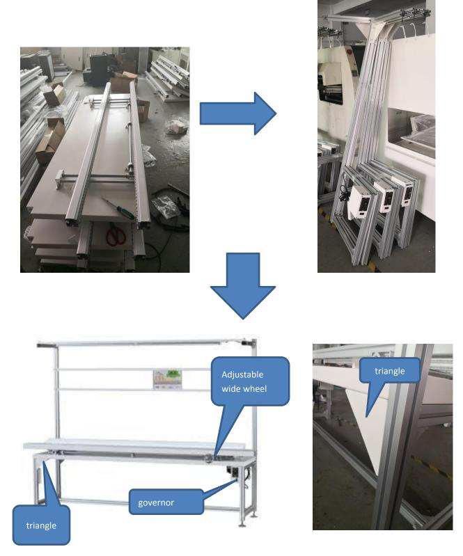
3. Install the foot connecting the aluminum with the lamp
