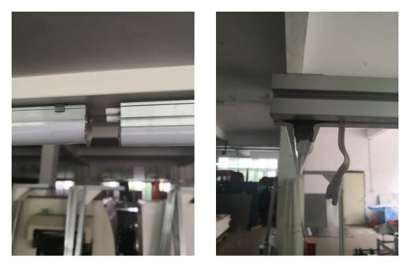
Installation of process card aluminum: install the process card aluminum between two aluminum brackets, adjust the appropriate height and spacing, so as to adapt to the placement of A4
