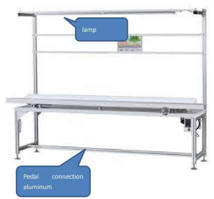
4.Installation of the transmission motor: install the transmission bevel gear onto the transmission motor, and use the rice screw to fix it tightly. Install the motor on the main platform before the motor is installed.Connect the motor power cord to the governor power cord plug.Install the gear guard.
